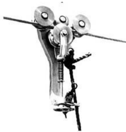
Fig. 5 - Ground connection of the OPGW cable at the tensioner outlet
