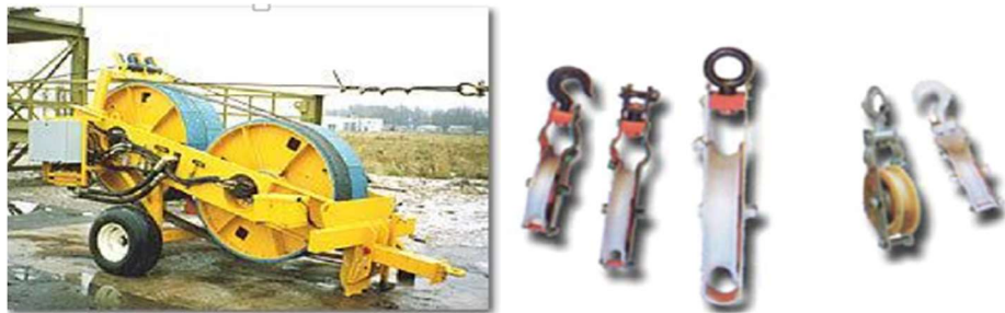
Figure 5 : Tensioner and stringing block
