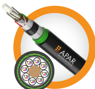
Loose Tube Double Jacket Steel Tape Armoured Cable Range: 12F-864F
