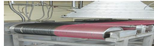
The cables are passed under the beam through a set of under beam equipment.
