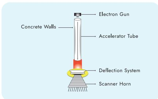
An Electron Gun is housed in a thick vessel where electrons are accelerated in an accelerator tube & directed to a scanning device magnetically to scan.
