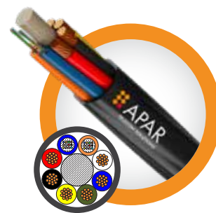
2-4 Core X 1.0 Sq.mm +1 - 48 F Microduct Hybrid Cable
