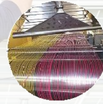
E-beam irradiated cables
