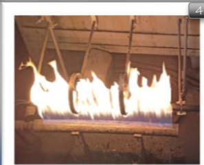
3 Oxygen Index test for power cable
