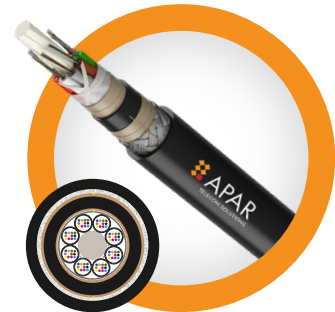
Loose Tube Double Jacket Braided Cable (750°C - 120 mins) OSP Range: 12F-96F
